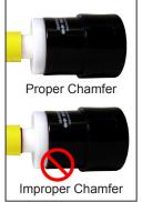
7 Stab pipe completely into fitting entrance.
